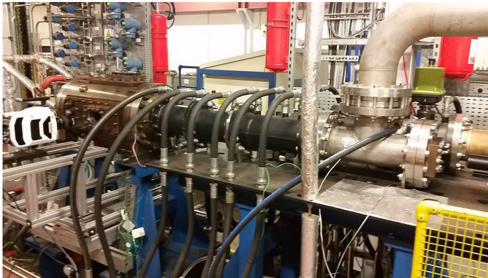
Rig for Steady-State Ammonia Spray Studies
