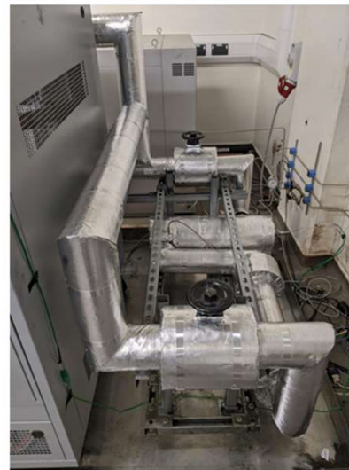
Demonstration of the Site Availability Model for MgH 2 system (150 g) with hot oil and electric heating and the hot oil system
