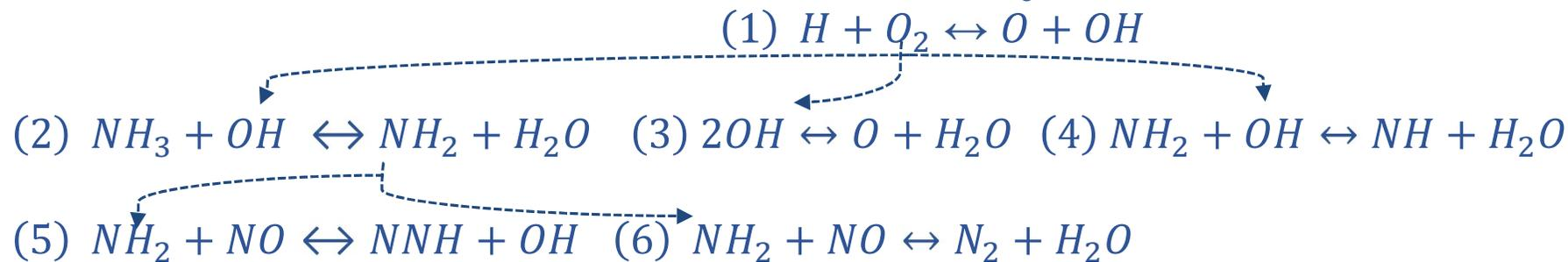
(1) & (5) increase flame temperatures, (6) inhibitor of temperature increase. As pressure increases, (3) is replaced with (4), whilst (7) competes with (1) and (8) for H species
