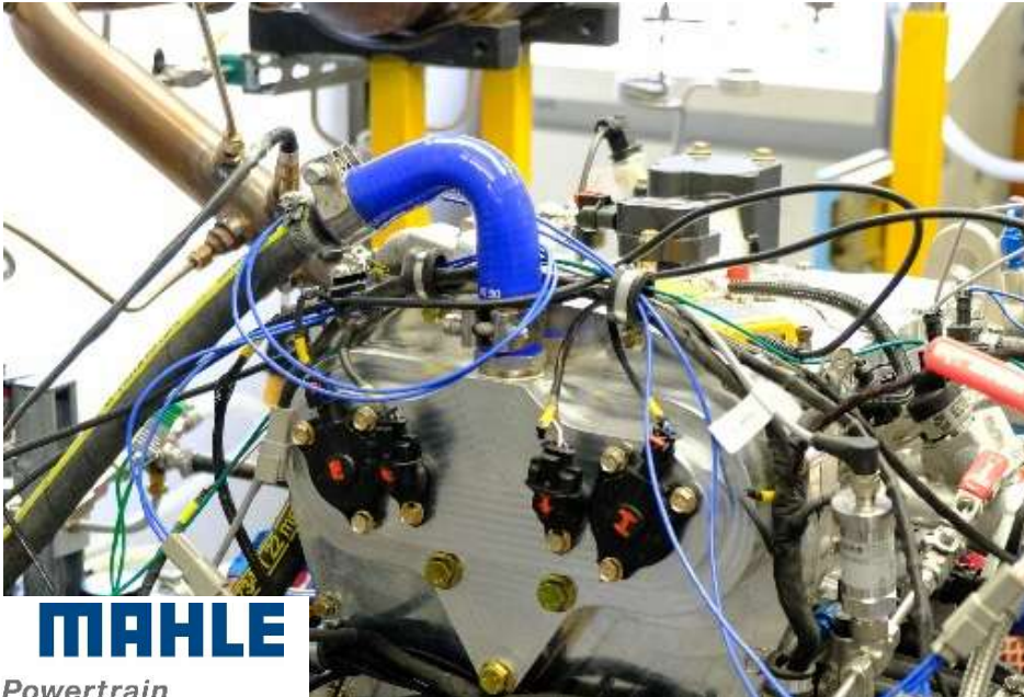
Single-Cylinder Research Engine (High Tumble) Compression Ratios: 12.5 and 17.5
